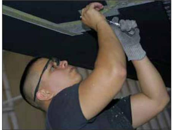
Senior Airman Arnold Carpio, MARS technician, scrapes old adhesive off the underside of an F-117A Nighthawk prior to laying down new radar-absorbent material.
