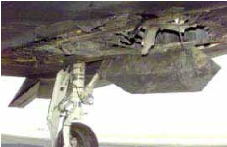
**F-117A 790 suffered extensive damage from an engine explosion and fire during a takeoff roll May 19, 1999.**
